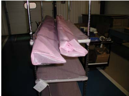
#3 – The panels are wrapped with foam and taped. Cardboard sleeves are attached to the leg extensions of each panel.
