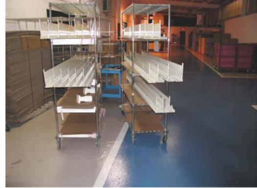
#2 – The components for each order are organized on moveable shelving racks. Each panel has a stamp for identification.
