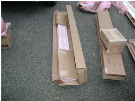
#5 – This is a finished two-panel box ready to be sealed. Panels are positioned back-to-back and secured with cardboard sleeves.
